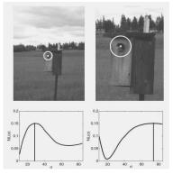
the ratio between the two characteristic scales is 2.64 similar to the actual scale factor of 2.59 relating the images
